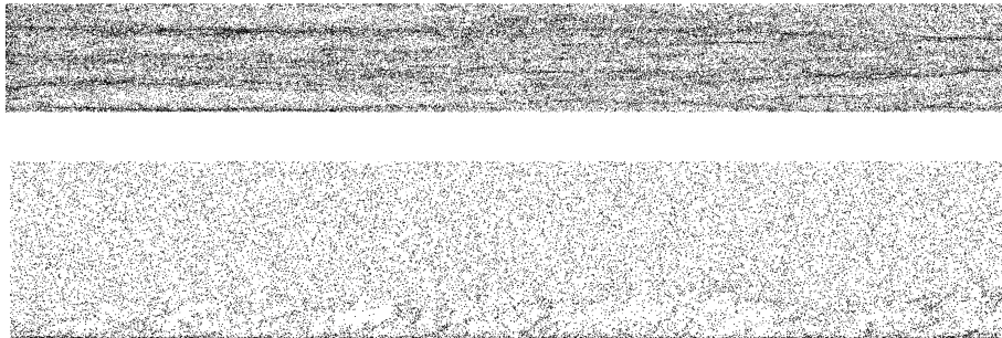
Figure: particle laden flow, compressible boundary layer, Re_{\delta_{99,e}} = 5000 , Ma = 0.8 , 512 \times 256 \times 128 , top: viscous sublayer in xz-plane; bottom: xy-plane
