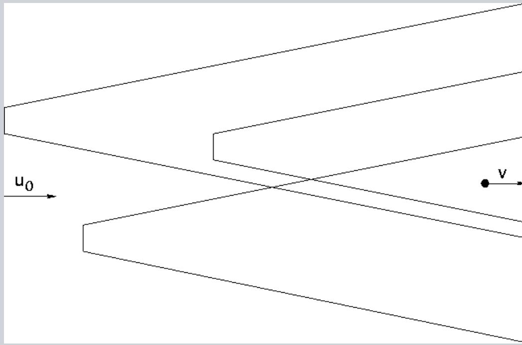
$$\left(1 - \frac{v}{u_0}\right)^2 = \left[\left(1 - \frac{v_1}{u_0}\right) \frac{A_1}{A_{\text{disc}}}\right]^2 + \left[\left(1 - \frac{v_2}{u_0}\right) \frac{A_2}{A_{\text{disc}}}\right]^2 + \dots$$
